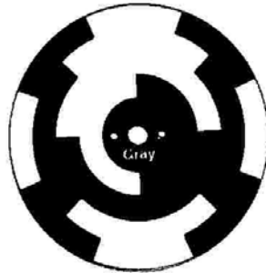
Figure 3. CE300 Gray code shaft encoder
