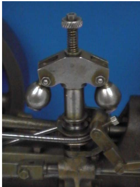
Figure 1. A Simple Centrifugal Speed Governor.
